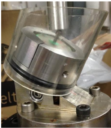
Figure 3-5.-Image of the final assembly of the implant tested inside the fatigue jaws.
