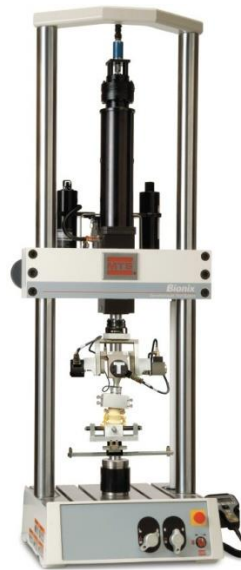
Figure 3-1.-Bionix-370 mechanical testing machine (MTS, USA) used for compression testing.
